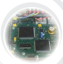
UHP-1000-CM is implemented as a compact single card ideal for integration into third-party OEM products. It is fully compatible with any other satellite routers of the UHP series. The router card has LED indicators, SMA or F type IF connectors and user LAN interface. Optionally, the router card can be equipped with the asynchronous LVTTL data port. Low power consumption and uniquely fast start upon power-up facilitate use of alternative power sources, such as solar batteries.
