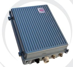
Rugged weatherproof satellite router UHP-1000-OD is designed for outdoor installation, for example, directly on the antenna. IP67 compliant enclosure and innovative system for active heating/cooling guarantees quick start and operating performance over a wide range of temperatures and a harsh environment. Supported power options include DC and Power over Ethernet (PoE).
